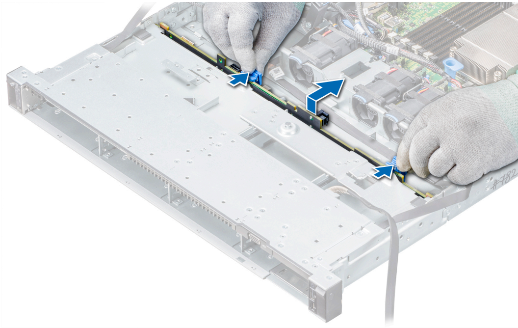
Figure 70. Removing the backplane
