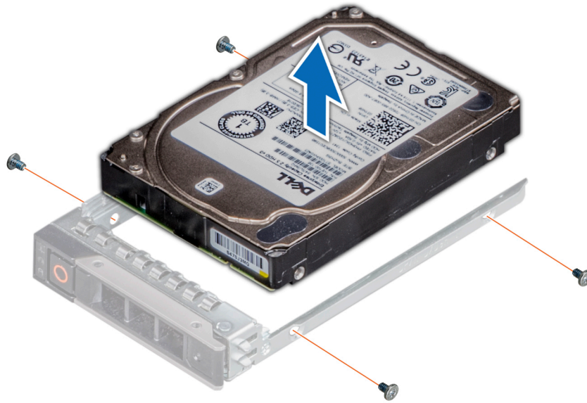
Figure 36. Removing the drive from the drive carrier
