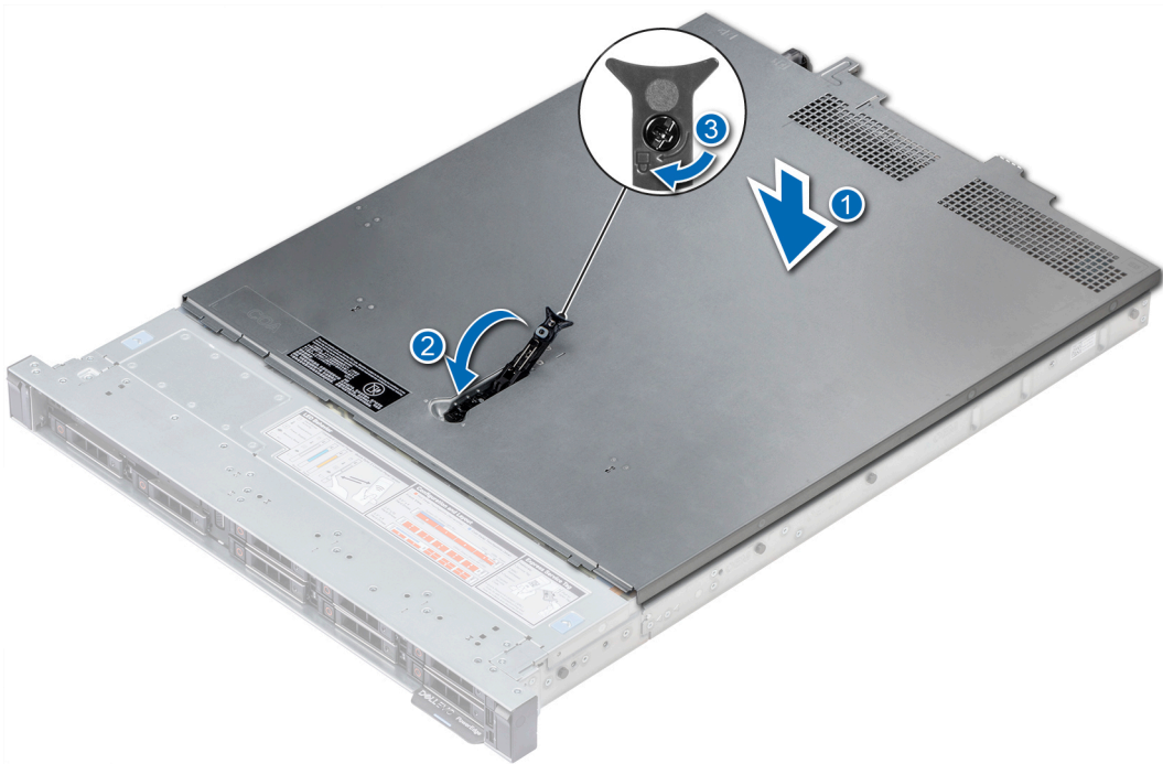
Figure 22. Installing system cover
