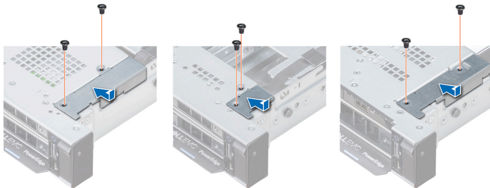
Figure 93. Installing the cable cover
