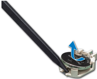
Figure 76. Removing the system battery
