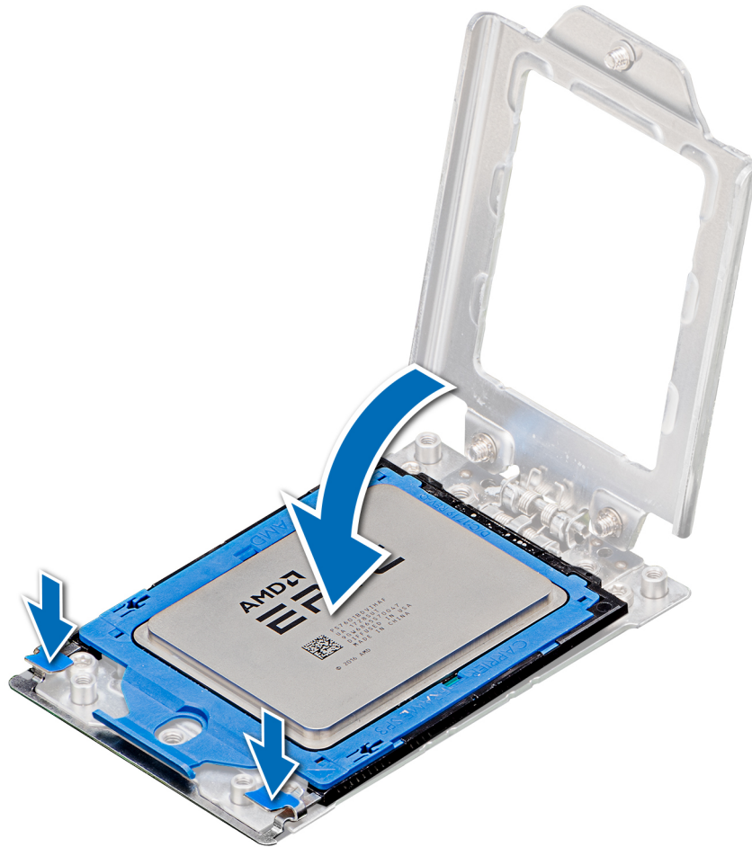
Figure 46. Closing the processor socket frame
